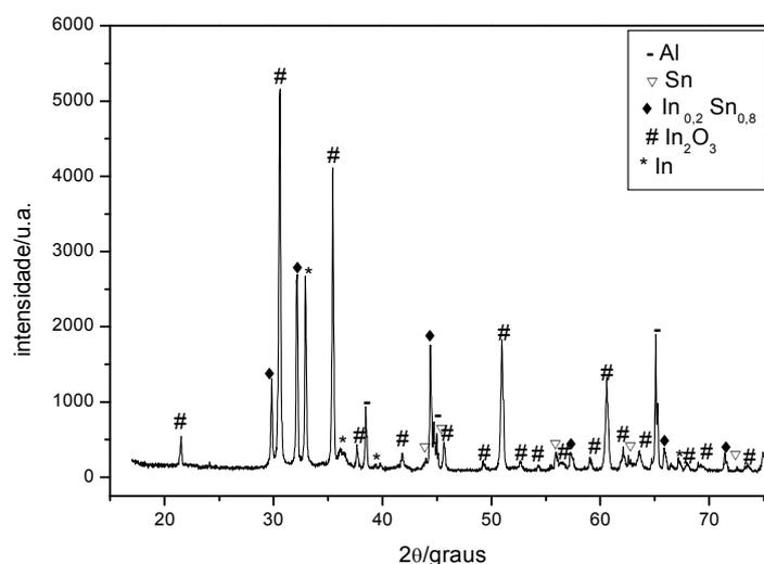
Figura 33: Difratograma de raios X do sistema 8 [ $\text{SnO}_2:\text{C}$  (1,5:1) e  $\text{In}_2\text{O}_3:\text{C}$  (1:1,5)].
