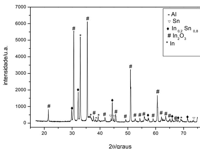
Figura 24: Difratograma de raios X do sistema 5 [ $\text{SnO}_2:\text{C}$  (1:1) e  $\text{In}_2\text{O}_3:\text{C}$  (1:1,5)].
