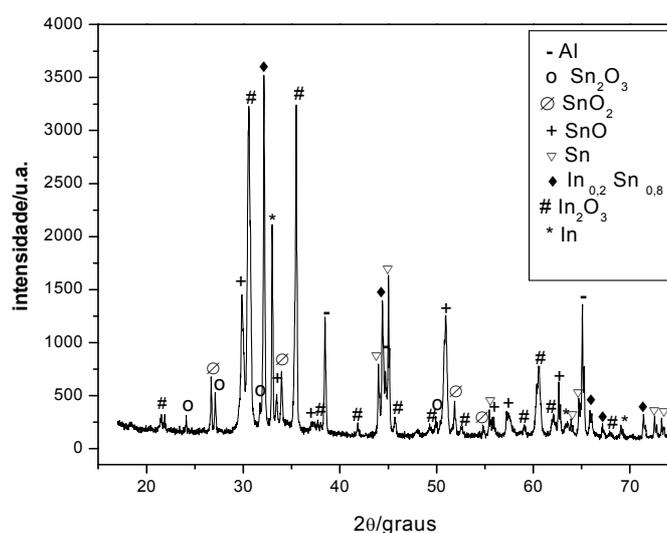
Figura 21: Difratograma de raios X do sistema 4 [ $\text{SnO}_2:\text{C}$  (1:1) e  $\text{In}_2\text{O}_3:\text{C}$  (1,5:1)].
