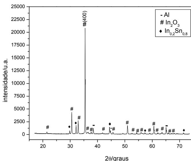
Figura 13: Difratograma de raios X do sistema 2 [ $\text{SnO}_2:\text{C}$  (1,5:1) e  $\text{In}_2\text{O}_3:\text{C}$  (1:1)].
