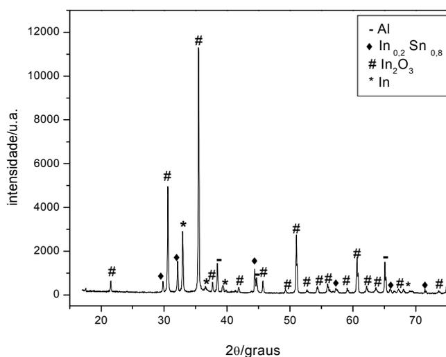
Figura 27: Difratograma do sistema 6 [ $\text{SnO}_2:\text{C}$  (1:1,5) e  $\text{In}_2\text{O}_3:\text{C}$  (1:1)].
