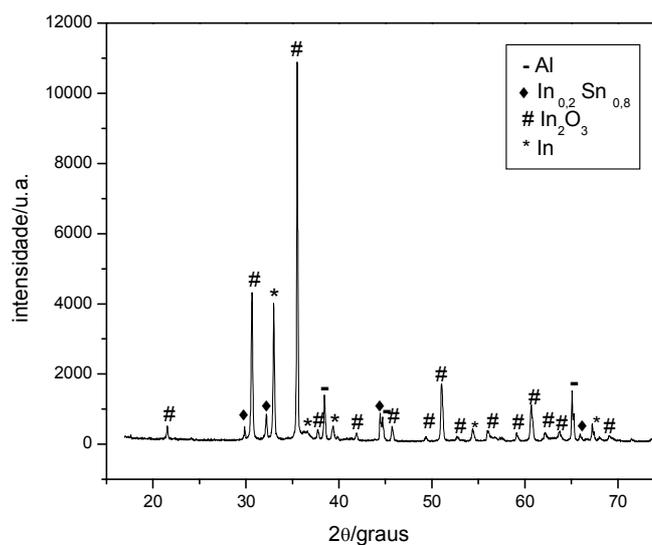
Figura 36: Difratograma de raios X do sistema 9 [ $\text{SnO}_2:\text{C}$  (1:1,5) e  $\text{In}_2\text{O}_3:\text{C}$  (1,5:1)].
