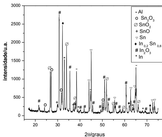
Figura 17: Difratoograma de raios X do sistema 3 [SnO<sub>2</sub>:C (1,5:1) e In<sub>2</sub>O<sub>3</sub>:C (1,5:1)].
