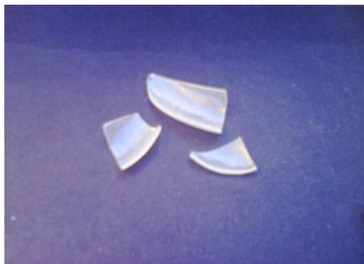
**Figura 8.** Amostra policristalina de SnO<sub>2</sub>:4%Eu.
