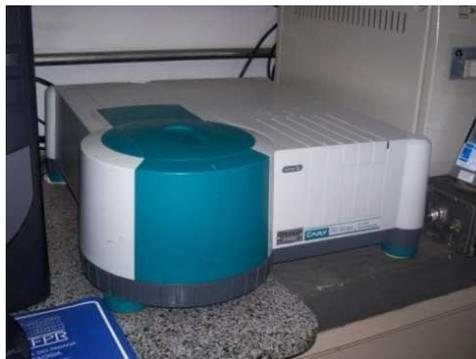
**FIGURA 3.3** – ESPECTROFOTÔMETRO UV/VIS.
