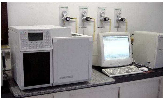
**FIGURA 3.2** – CROMATÓGRAFO CG – FID.
