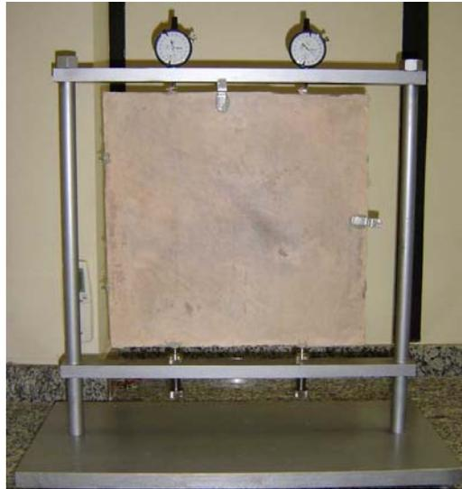
Figure 3. Drying shrinkage test set-up. The strains were measured by two strain indicators located at the top of the frame.
