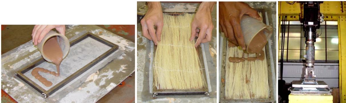
Figure 6 - Composite molding process.
