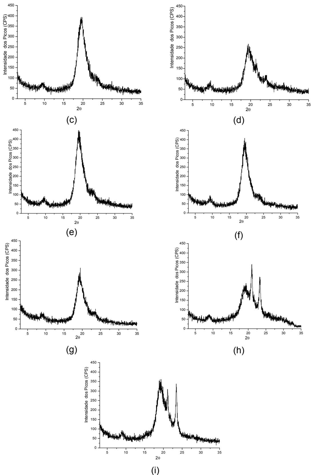
Figura 33 – Difratoograma de raios X de PU (a) e de quitina (b) e das blends PU/QTN: (c) 10/90, (d) 20/80, (e) 30/70, (f) 40/60, (g) 50/50, (h) 60/40 e (i)70/30.
