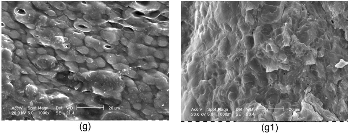
Figura 49 - Micrografia das blendas: (a) 10/90, (b) 20/80, (c) 30/70, (d) 40/60, (e) 50/50, (f) 60/40, (g) 70/30 e (a1), (b1), (c1), (d1), (e1), (f1), (g1) suas respectivas fraturas.
