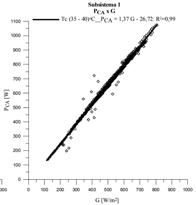
(d)  $P_{CA}$  para  $T_m (35 - 40) ^\circ C$ .
