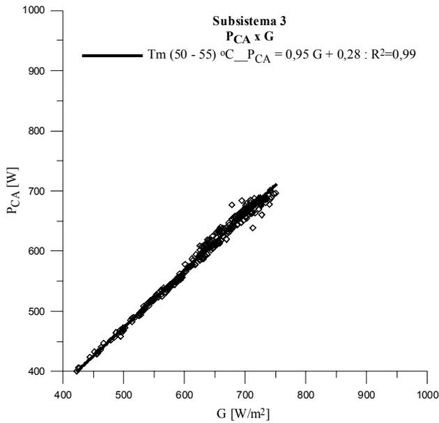
(g)  $P_{CA}$  para  $Tm (50 - 55) \text{ } ^\circ\text{C}$ .
