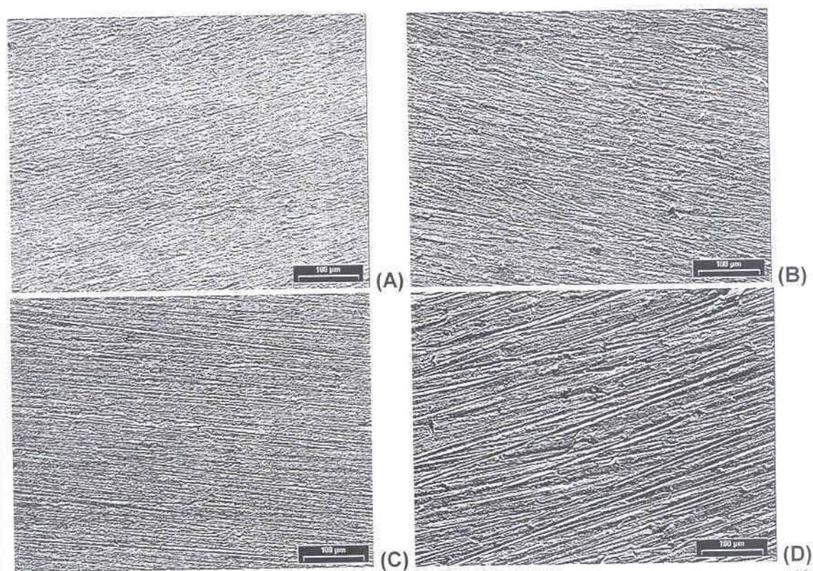
FIGURA 73 – ASPECTO SUPERFICIAL DAS PONTAS DE COBRE, POLIMENTO MECÂNICO: (A) LIXA 2000, (B) LIXA 1500, (C) LIXA 1000 E (D) LIXA 600 – VISTA GERAL (AUMENTO 200 X)
