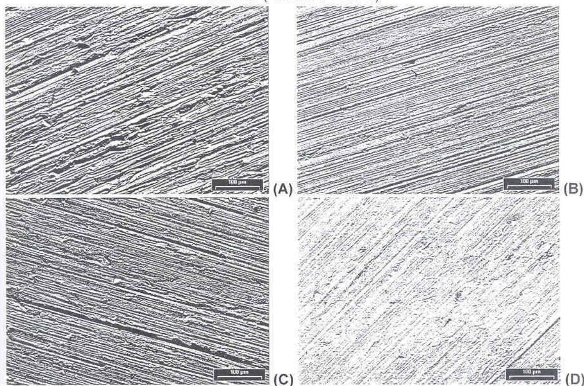
FIGURA 78 – ASPECTO SUPERFICIAL DAS PONTEIRAS DE COBRE APÓS PASSIVAÇÃO,  $E_{\text{DEP}}$ : - 930 mV, LIXA 600,  $Q_{\text{DEP}}$ : (A) 5 mC, (B) 15 mC, (C) 35 mC E (D) 80 mC – VISTA GERAL (AUMENTO 200 X)
