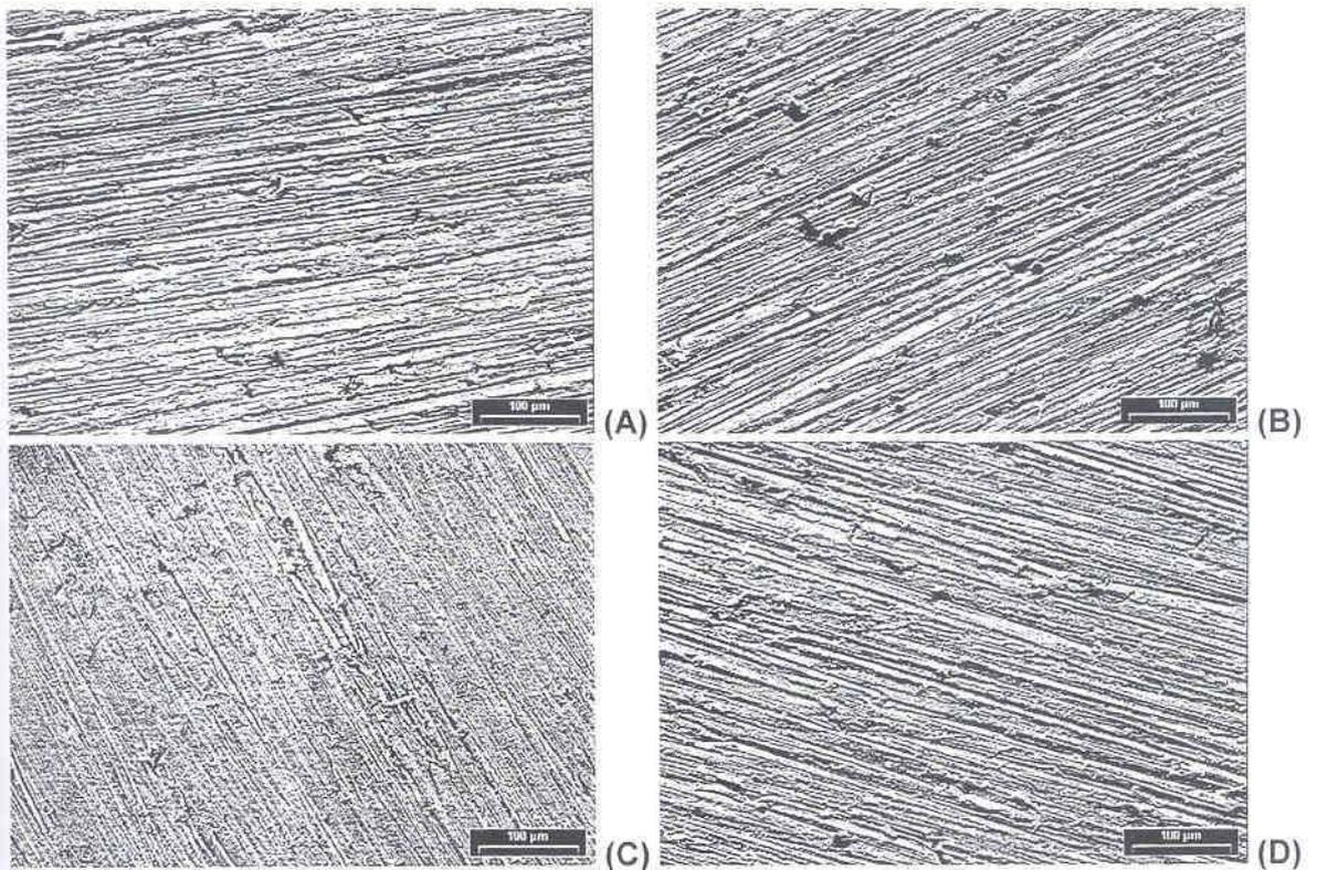
FIGURA 76 – ASPECTO SUPERFICIAL DAS PONTEIRAS DE COBRE APÓS PASSIVAÇÃO,  $E_{\text{DEP}}: -830 \text{ mV}$ , LIXA 600,  $Q_{\text{DEP}}: (A) 5 \text{ mC}$ , (B) 15 mC, (C) 35 mC E (D) 80 mC – VISTA GERAL (AUMENTO 200 X)
