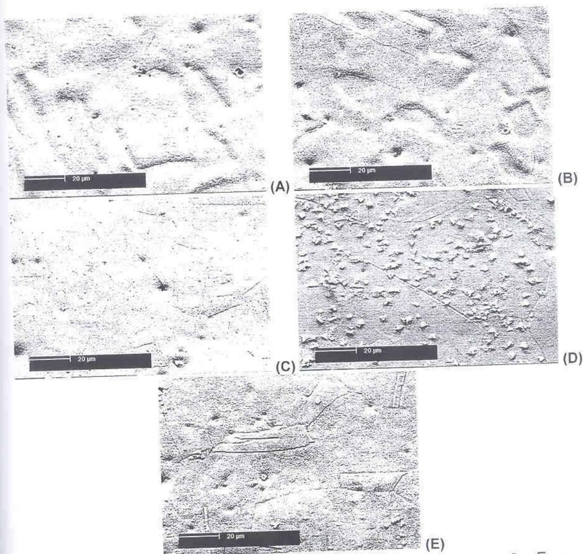
FIGURA 83 – ASPECTO SUPERFICIAL DAS PONTEIRAS DE COBRE APÓS PASSIVAÇÃO,  $E_{\text{DEP}}$ : -930 mV, POLIMENTO QUÍMICO,  $Q_{\text{DEP}}$ : (A) 5 mC, (B) 15 mC, (C) 25 mC, (D) 35 mC E (E) 80 mC – DETALHE DO CENTRO (AUMENTO 1000 X)
