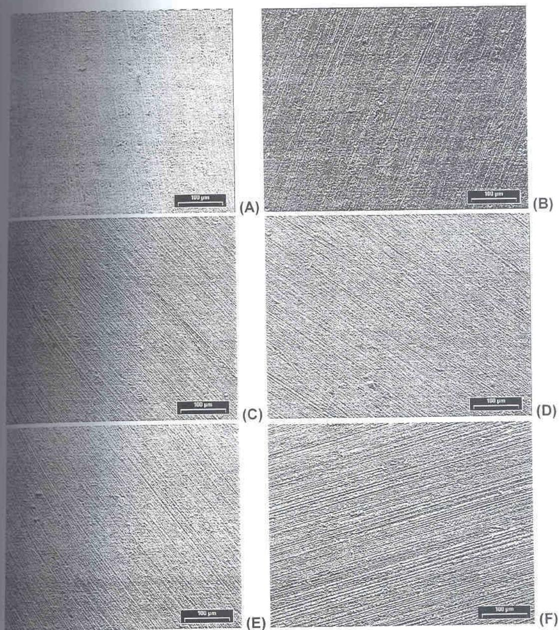
FIGURA 71 – ASPECTO SUPERFICIAL DAS PONTEIRAS DE COBRE APÓS PASSIVAÇÃO,  $E_{DEP}$ : -930 mV, LIXA 2000,  $Q_{DEP}$ : (A) 5 mC, (B) 15 mC, (C) 25 mC, (D) 35 mC, (E) 50 mC E (F) 80 mC – VISTA GERAL (AUMENTO 200 X)
