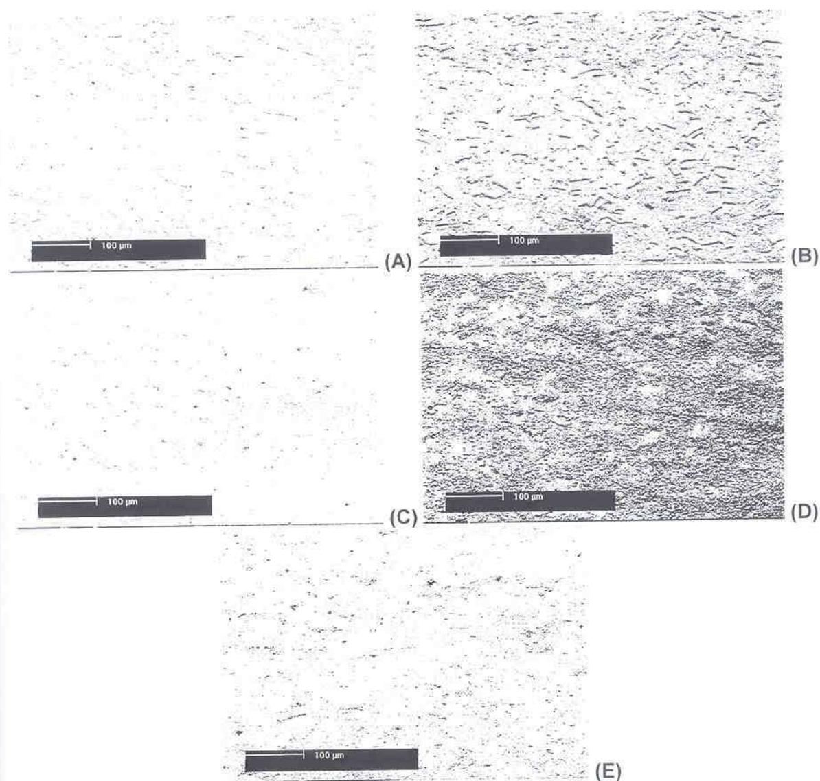
FIGURA 82 – ASPECTO SUPERFICIAL DAS PONTEIRAS DE COBRE APÓS PASSIVAÇÃO,  $E_{\text{DEP}}: -930 \text{ mV}$ , POLIMENTO QUÍMICO,  $Q_{\text{DEP}}: (A) 5 \text{ mC}, (B) 15 \text{ mC}, (C) 25 \text{ mC}, (D) 50 \text{ mC}$  E (E)  $80 \text{ mC}$  – VISTA GERAL (AUMENTO 200 X)
