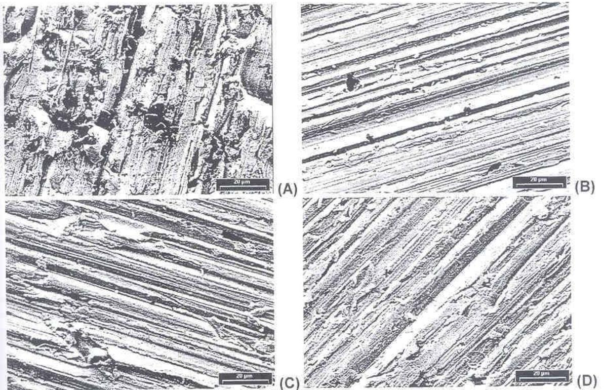
FIGURA 79 – ASPECTO SUPERFICIAL DAS PONTEIRAS DE COBRE APÓS PASSIVAÇÃO,  $E_{\text{DEP}} = -930 \text{ mV}$ , LIXA 600,  $Q_{\text{DEP}}$ : (A) 5 mC, (B) 15 mC, (C) 35 mC E (D) 80 mC – DETALHE DA BORDA (AUMENTO 1000 X)
