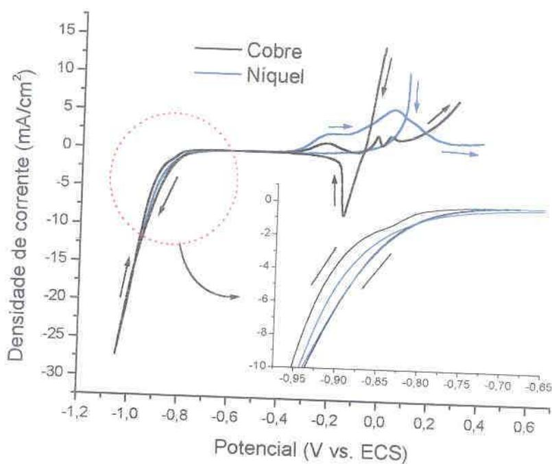
FIGURA 38 – VOLTAMETRIA PARA OS ELETRODOS DE COBRE E NÍQUEL NA SOLUÇÃO DE WATTS SEM ADITIVOS ORGÂNICOS, VV: 10 mV/s
