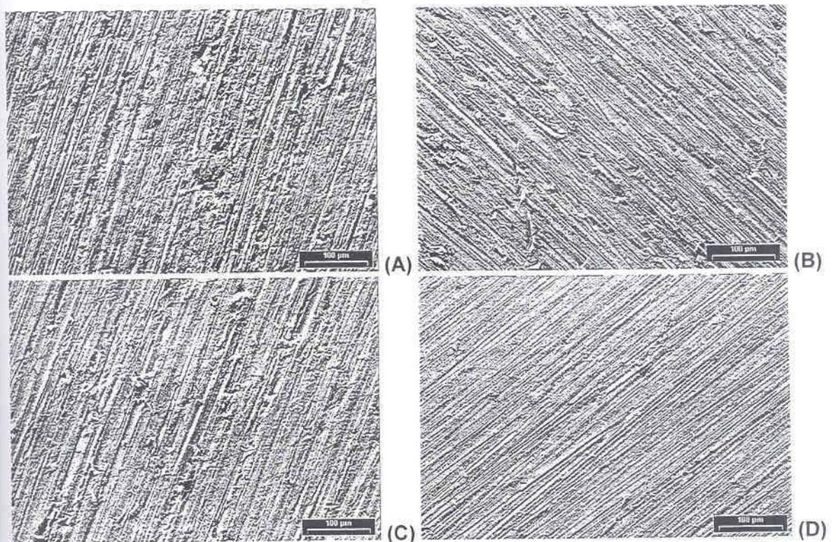
FIGURA 80 – ASPECTO SUPERFICIAL DAS PONTEIRAS DE COBRE APÓS PASSIVAÇÃO,  $E_{\text{DEP}} = -1030 \text{ mV}$ , LIXA 600,  $Q_{\text{DEP}}$ : (A) 5 mC, (B) 15 mC, (C) 35 mC E (D) 80 mC – VISTA GERAL (AUMENTO 200 X)
