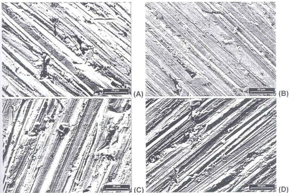
FIGURA 81 – ASPECTO SUPERFICIAL DAS PONTEIRAS DE COBRE APÓS PASSIVAÇÃO,  $E_{\text{DEP}}$ : -1030 mV, LIXA 600,  $Q_{\text{DEP}}$ : (A) 5 mC, (B) 15 mC, (C) 35 mC E (D) 80 mC – DETALHE DO CENTRO (AUMENTO 1000 X)
