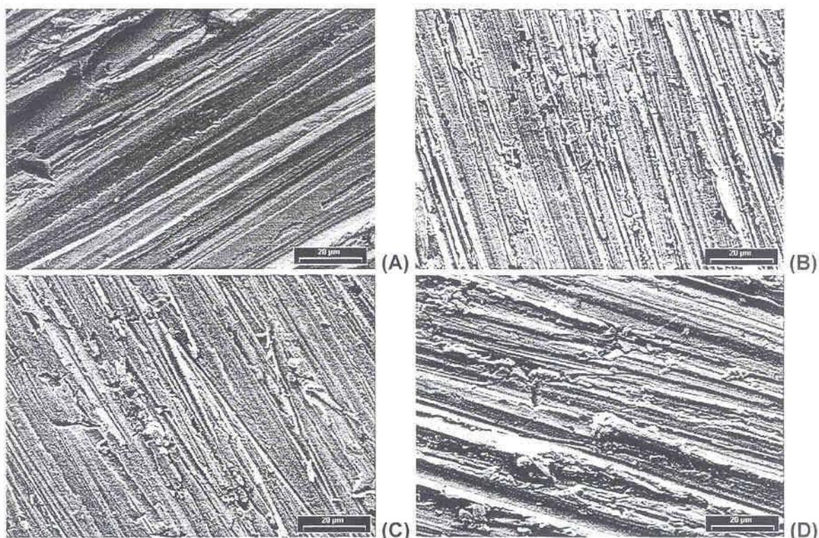
FIGURA 77 – ASPECTO SUPERFICIAL DAS PONTEIRAS DE COBRE APÓS PASSIVAÇÃO,  $E_{\text{DEP}}$ : - 830 mV, LIXA 600,  $Q_{\text{DEP}}$ : (A) 5 mC, (B) 15 mC, (C) 35 mC E (D) 80 mC – DETALHE DO CENTRO (AUMENTO 1000 X)
