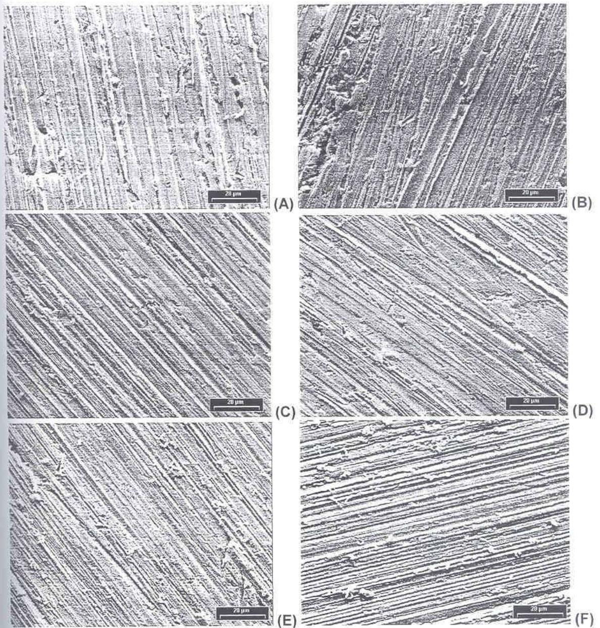
FIGURA 72 – ASPECTO SUPERFICIAL DAS PONTEIRAS DE COBRE APÓS PASSIVAÇÃO,  $E_{\text{DEP}}$ : - 930 mV, LIXA 2000,  $Q_{\text{DEP}}$ : (A) 5 mC, (B) 15 mC, (C) 25 mC, (D) 35 mC, (E) 50 mC E (F) 80 mC – DETALHE DO CENTRO (AUMENTO 1000 X)
