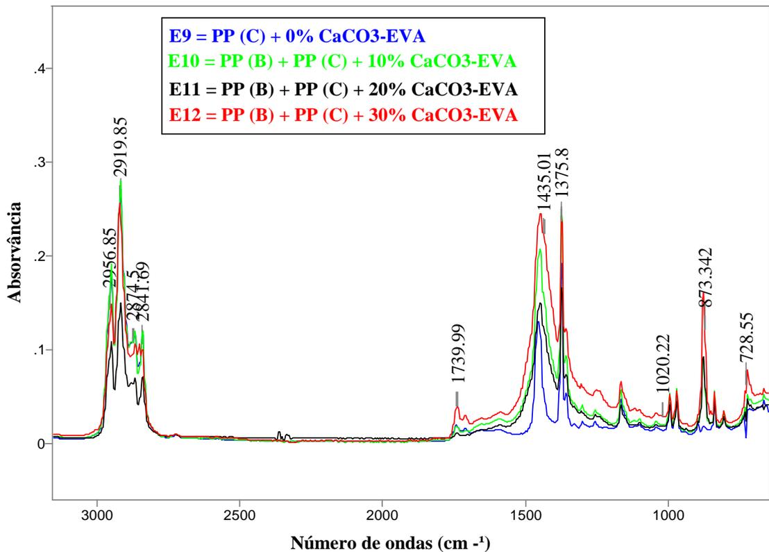
**Figura 6.11** Espectro IR do PP (B) + PP (C) + CaCO<sub>3</sub>-EVA - Ensaios (9 a 12).
