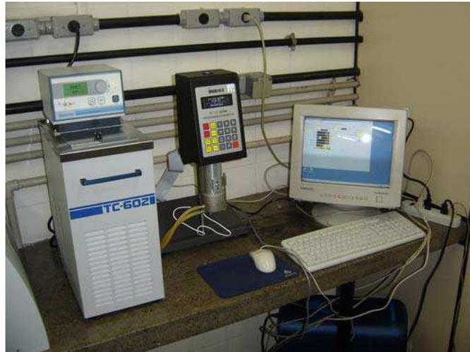
**Figura III.18 - Reômetro LVDV-IIIU operando no LTTC.**
