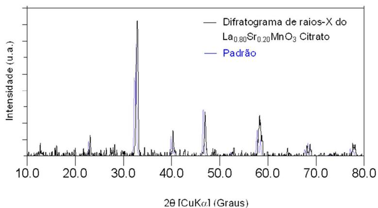
Figura 3.1. Difratoograma do pó de  $\text{La}_{0.8}\text{Sr}_{0.2}\text{MnO}_3$  citrato.
