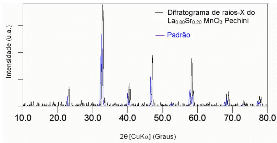
Figura 3.3. Difratoograma do pó de  $\text{La}_{0.8}\text{Sr}_{0.2}\text{MnO}_3$  pechini.
