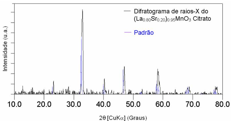
Figura 3.2. Difratoograma do pó de  $(\text{La}_{0.8}\text{Sr}_{0.2})_{0.95}\text{MnO}_3$  citrato.
