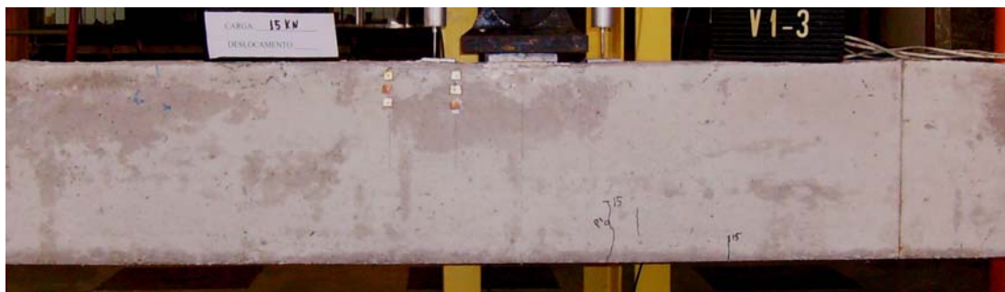
(a) P = 15,0 \text{ kN} ( \sim 1,03 P_{cr} e 40\% P_u ).
