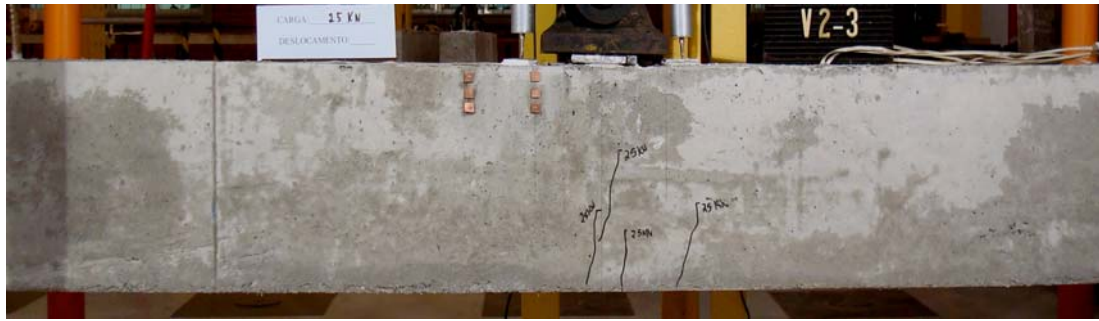
(a) P = 25,0 \text{ kN} ( \sim 1,60 P_{cr} e 45\% P_u ).
