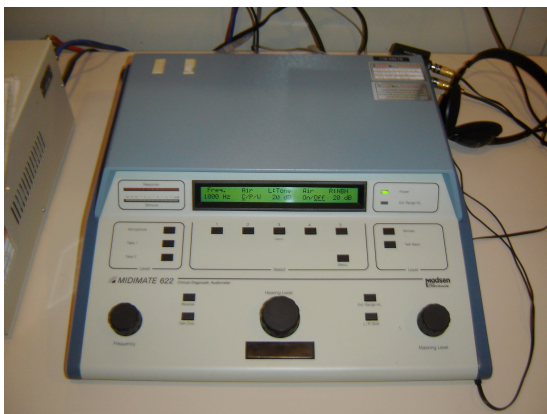
Figura 2 - Audiômetro (Midimate 622, Madsen Eletronics)
