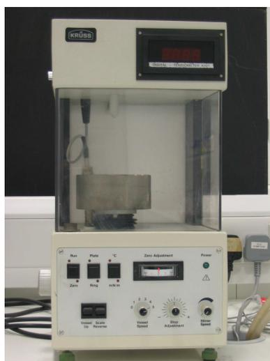
Figura 24 – Tensiômetro digital K10ST
