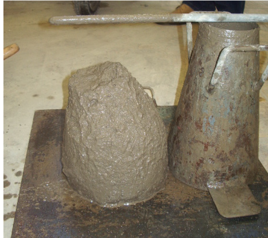
Foto 5.3 – Concreto no traço 1:5,0 com teor de argamassa igual a 54%
