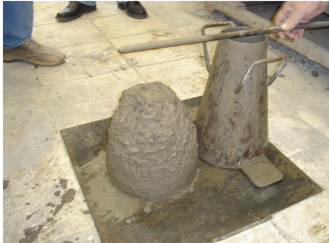
Foto 6.5 – Slump – traço 1:5,0 – 5% RBMG
