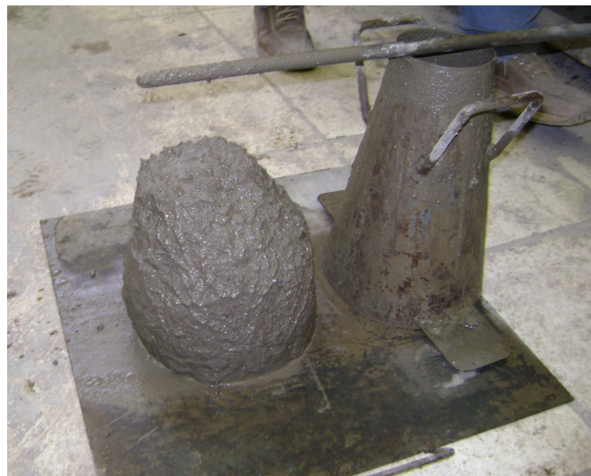
Foto 6.6 – Slump – traço 1:5,0 – 10% RBMG
