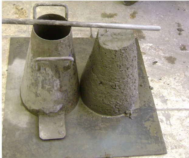
Foto 6.8 – Slump – traço 1:5,0 – 20% RBMG
