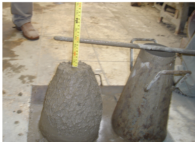
Foto 6.7 – Slump – traço 1:5,0 – 15% RBMG
