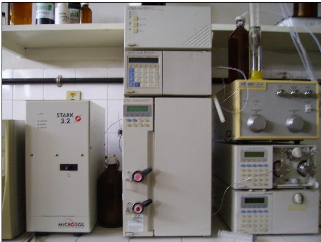
**Figura 6 – HPLC (High Performance Liquid Cromatography)**
