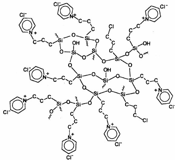
**Figura 18:** Estrutura do policátion  $\text{SiPy}^+\text{Cl}^-$
