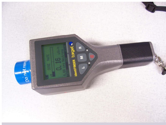
FIG. 2.6 IndentiFINDER, modelo 21305 do Fabricante Thermo Electron Corporation.
