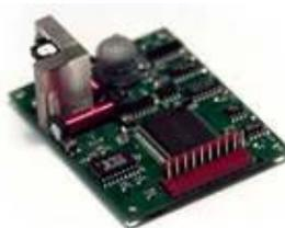
**Figura 3-7: CPS (Roll, Pitch, Yaw e Campo Magnético).**
