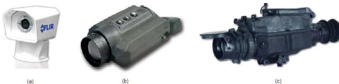
FIG. 1.26 – (a) Câmera SR-19 (FLIR, 2008); (b) hand-held thermal imager (DRS, 2008); (c) thermal weapon sight (RAYTHEON, 2008).
