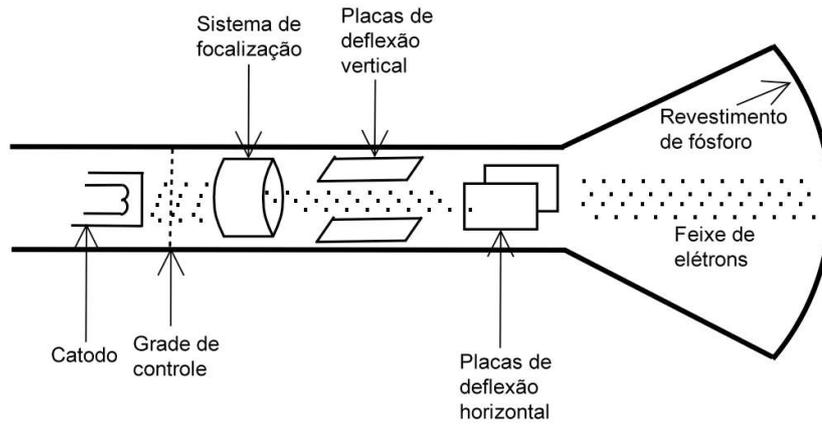
Figura 19: Cathode Ray Tube (CRT).
