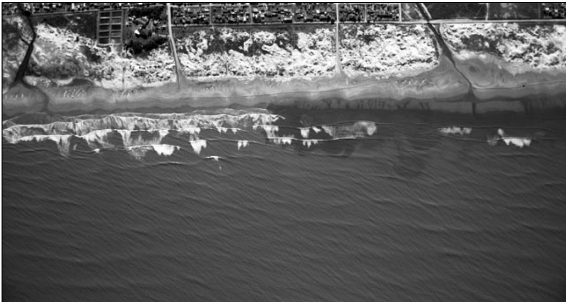
Figure 5. 2 - A) Morphology of the inner continental shelf adjacent to the Patos Lagoon inlet where mud is deposit (Calliari et al. 2007). B) Lateral variability in wave breaking and clear wave damping, associated with the presence of mud.
