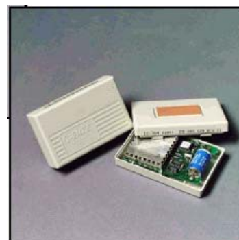
Fig. 3.5.d – MD5803 R/W Q-FREE TAG R/W
