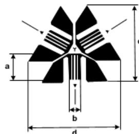
Figura A.10: Extensômetro triaxial a  $120^\circ$  (ECXELSENSOR, 2007).
