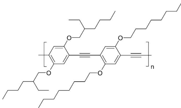
PPDPV  $\mu_e = 4,0 \times 10^{-4} \text{ cm}^2\text{V}^{-1}\text{s}^{-1}$
