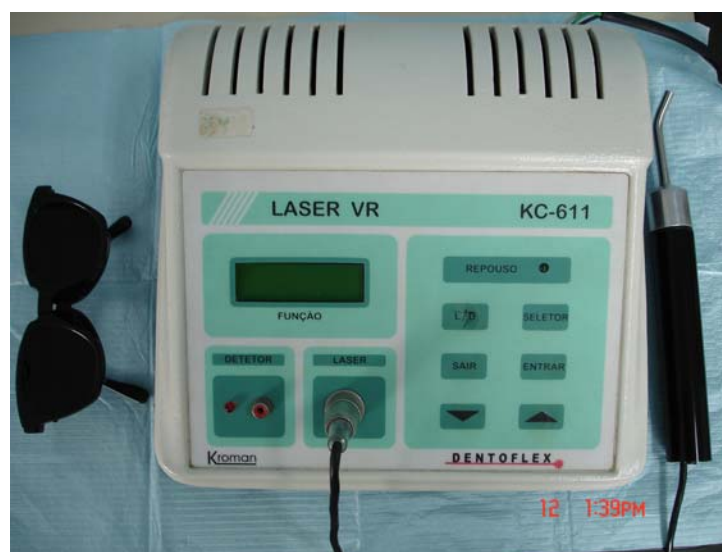
Figura 1 – Laser AlGaAs (670 nm)
