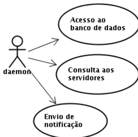
Figura 4.25: Casos de uso do *daemon* "Job Monitor"
