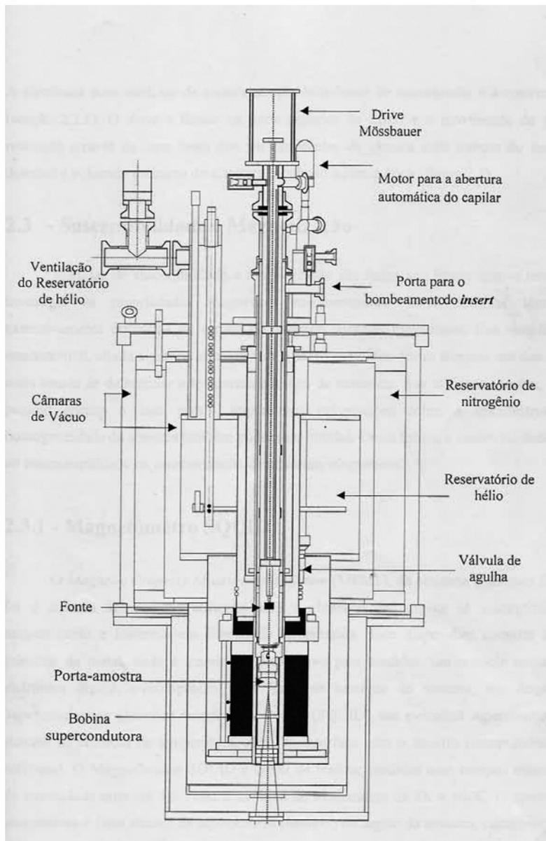
**Figura 3.3:** Criostato Oxford – Superconducting Magnet system[13].
