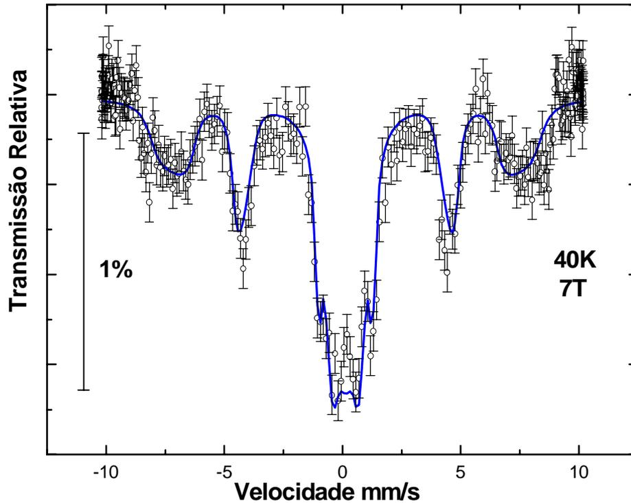
Figura 4.25. Espectro Mössbauer de  $\text{NdNi}_{0.99}\text{Fe}_{0.01}\text{O}_3$ , medidos com  $B_{\text{EXT}}=7\text{T}$  a  $40\text{K}$ .
