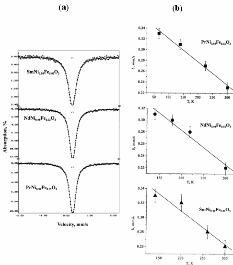
**Figura 2.21.** (a) EM do  $^{57}\text{Fe}$  no  $\text{RNi}_{0.98}\text{Fe}_{0.02}\text{O}_3$  ( $\text{R}=\text{Nd, Sm, Pr}$ ) a 300 K. (b) Deslocamento isomérico do  $^{57}\text{Fe}$  no  $\text{RNi}_{0.98}\text{Fe}_{0.02}\text{O}_3$  ( $\text{R}=\text{Nd, Sm, Pr}$ ) em função da temperatura [56].
