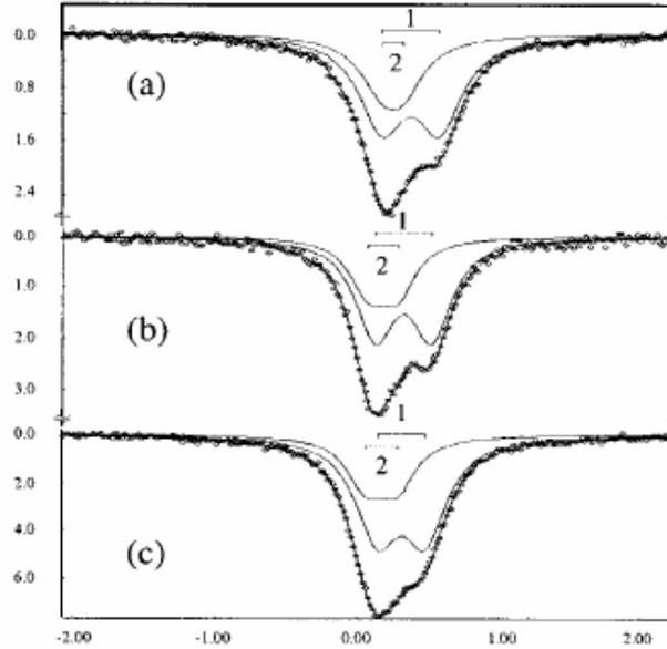
**Figure 2.19.** Espectros mössbauer para 300 K do (a)  $\text{TlNi}_{0.98}\text{Fe}_{0.02}\text{O}_3$  (b)  $\text{LuNi}_{0.98}\text{Fe}_{0.02}\text{O}_3$ , and (c)  $\text{YNi}_{0.98}\text{Fe}_{0.02}\text{O}_3$ . (1 = Fe(1), 2=Fe(2))
