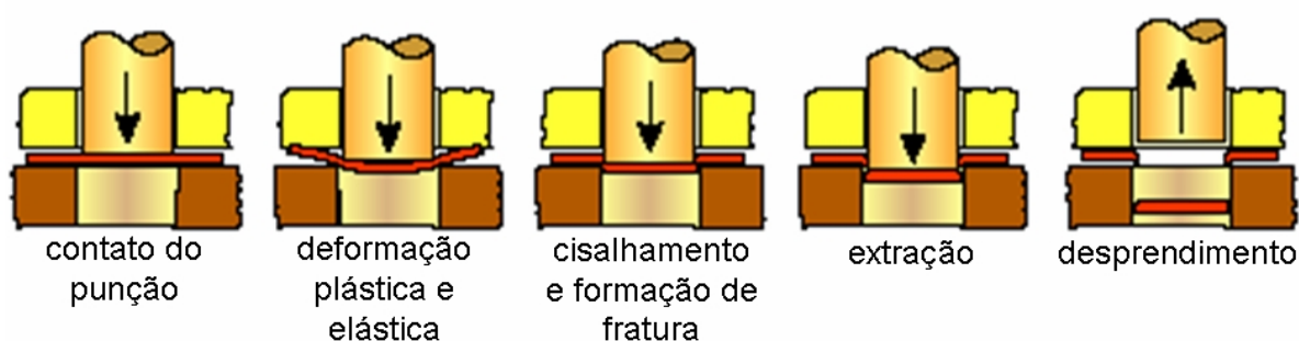
Figura 3.4.7 – As fases do processo de blanking (SCHULER, 1998).
