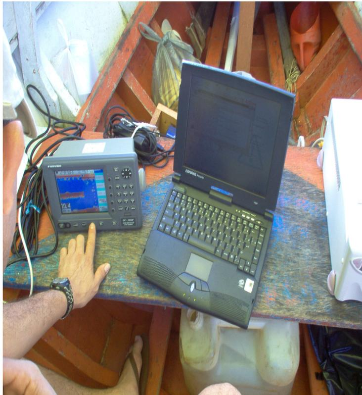
Figura 30: A Ecossonda DGPS/PLOTTER/SONAR, com visor colorido FURUNO GP-1850 F e o notebook.
