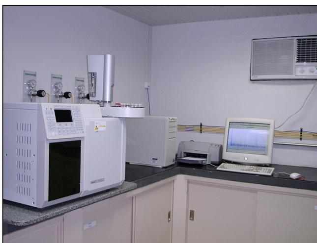
FIGURA 09 – CROMATÓGRAFO A GÁS VARIAN, MODELO CP 3800 COM DETECTOR FID
