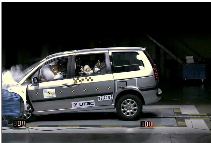
Figura 19: Peugeot 807 * - Front impact, (EURONCAP, 2002).
