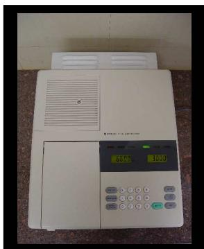
3. Espectrofômetro (Hitachi® U-1100 Spectrophotometer)
