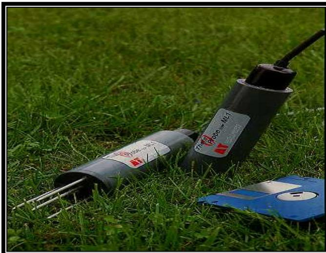
Figura 6.11: Sonda Theta ML2 (Delta – T Devices, UK, 2000).
