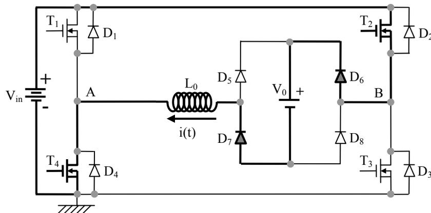
Figura 2.11: Intervalo  $\Delta t_6 = [t_5, t_6]$
