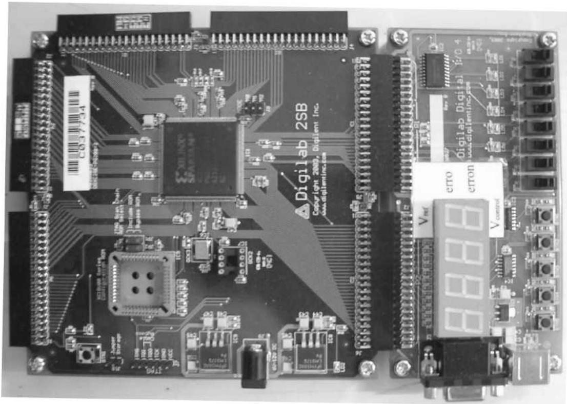
Figura 5.12: Placa de circuito D2SB com FPGA SPARTAN XC2S200E.
