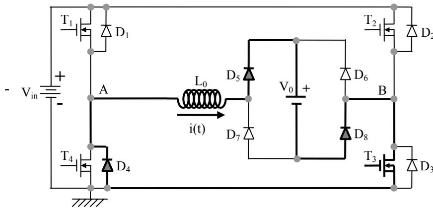
Figura 2.9: Intervalo  $\Delta t_4 = [t_3, t_4]$
