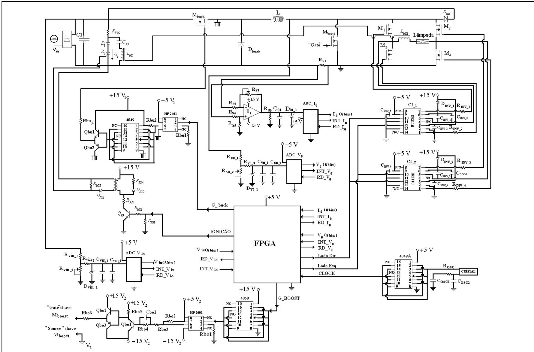
**REATOR ELETRÔNICO UTILIZANDO O CONVERSOR “BUCK+BOOST” EM CASCATA**
