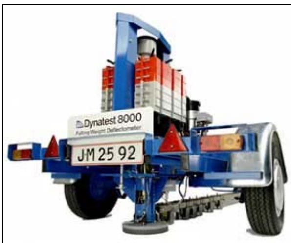
Figura 3.8 – Dynatest FWD 8000 ( www.dynatest.com/hardware/fwd_hwd.htm ) acesso em 22/11/05.
