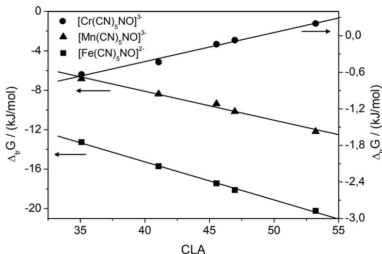
**Figura 32.** Energia livre de Gibbs de transferência versus CLA para os ânions complexos:  $[\text{Cr}(\text{CN})_5\text{NO}]^{3-}$  (●),  $[\text{Mn}(\text{CN})_5\text{NO}]^{3-}$  (▲) e  $[\text{Fe}(\text{CN})_5\text{NO}]^{2-}$  (■), no SAB  $\text{Li}_2\text{SO}_4/\text{PEO4000}/\text{H}_2\text{O}$  a 25 °C.
