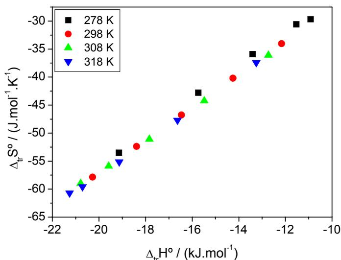
**Figura 23.**  $\Delta_{tr}S^\circ$  versus  $\Delta_{tr}H^\circ$  para o complexo  $[\text{Mn}(\text{CN})_5\text{NO}]^{3-}$  em SAB's PEO/ $\text{Na}_2\text{SO}_4/\text{H}_2\text{O}$  nas temperaturas: 278 K (■), 298 K (●), 308 K (▲), 318 K (▼).
