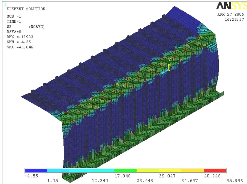
FIG. 4.40 – Tensões  $\sigma_z$  para reação de 45,30 kN
