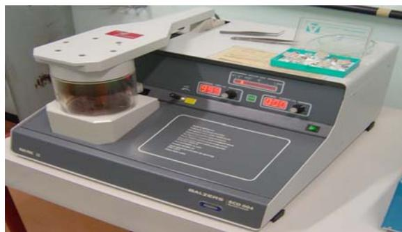
**FIGURA 14** – Aparelho *Sputtercoating EMITECH K 550*.
