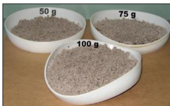
Figure 4. Fermented products obtained in sieves with 50, 75 and 100 g of substrate (dry basis).
