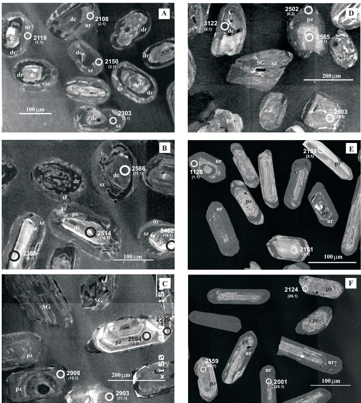
**Figure 5-** Cathodoluminescence images of analyzed zircon crystals of the samples MVD21 (A and B), MVD40 (C and D) and MVD34A (E and F), with the ion microprobe spots and their their number in the parentheses and respective  $^{207}\text{Pb}/^{206}\text{Pb}$  ages. Detail of detrital cores (dc), planar (pz) and sector (sz) zoning, dark (dr) and unzoned (ur) rims, sealed fractures (sf) and striated grains (SG).
