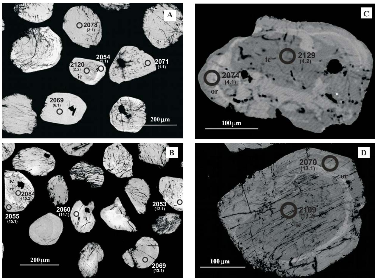
**Figure 9-** Backscattered electron images of analyzed monazite crystals of the samples MVD26B (A and B) and MVD34A (C and D), with the ion microprobe spots their number in the parentheses and respective  $^{207}\text{Pb}/^{206}\text{Pb}$  ages. Detail of inherited cores (ic) and overgrowth rims (or).
