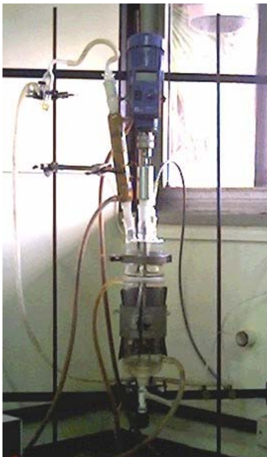
Figure 20. Pyrex glass reactor (1.0 L) used for reactor blends production.
