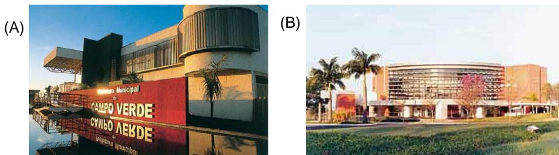
FIGURA 18 – Exemplo de *brise-soleil* vertical (A) e horizontal (B)
