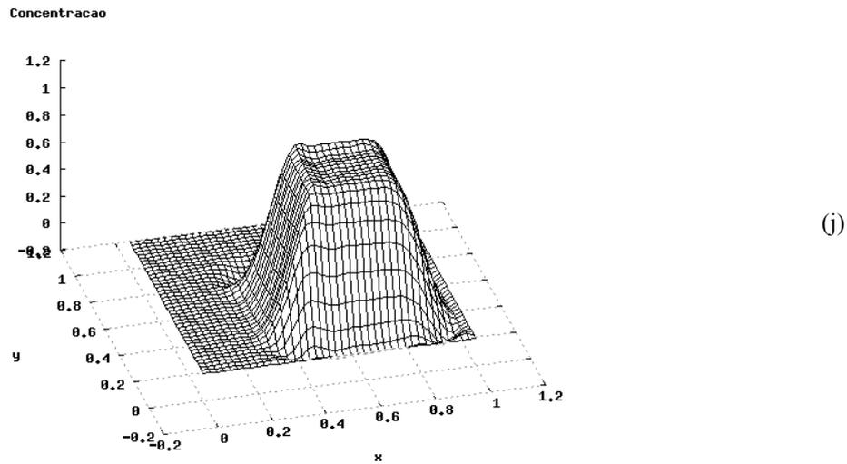
**Figura 4.33** Platô em movimento diagonal, quadrilátero bi-linear com integração reduzida, passo de tempo 29, (a) *SUPG*,  $\varepsilon=0.0$ ; (b) *SUPG*,  $\varepsilon=1.0$ ; (c) *CAU*,  $\varepsilon=0.0$ ; (d) *CAU*,  $\varepsilon=0.05$ ; (e) *CD*,  $\varepsilon=0.0$ ; (f) *CD*,  $\varepsilon=0.05$ ; (g) *ETV*,  $\varepsilon=0.0$ ; (h) *ETV*,  $\varepsilon=1.0$ ; (i) *ASGS*,  $\varepsilon=0.0$ ; (j) *ASGS*,  $\varepsilon=0.05$ .
