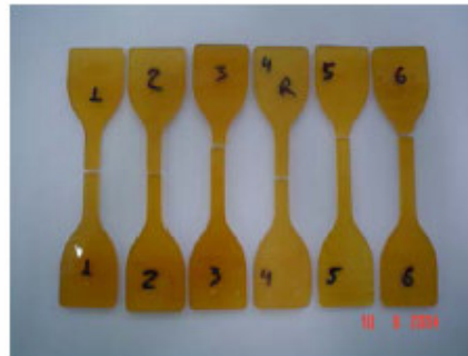
Figure 3. Samples used to determine the resin's modulus of elasticity.
