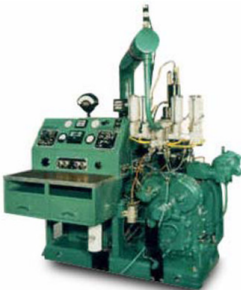
Figura IV.8 – Motor CFR instalado no SENAI/CETIND.
