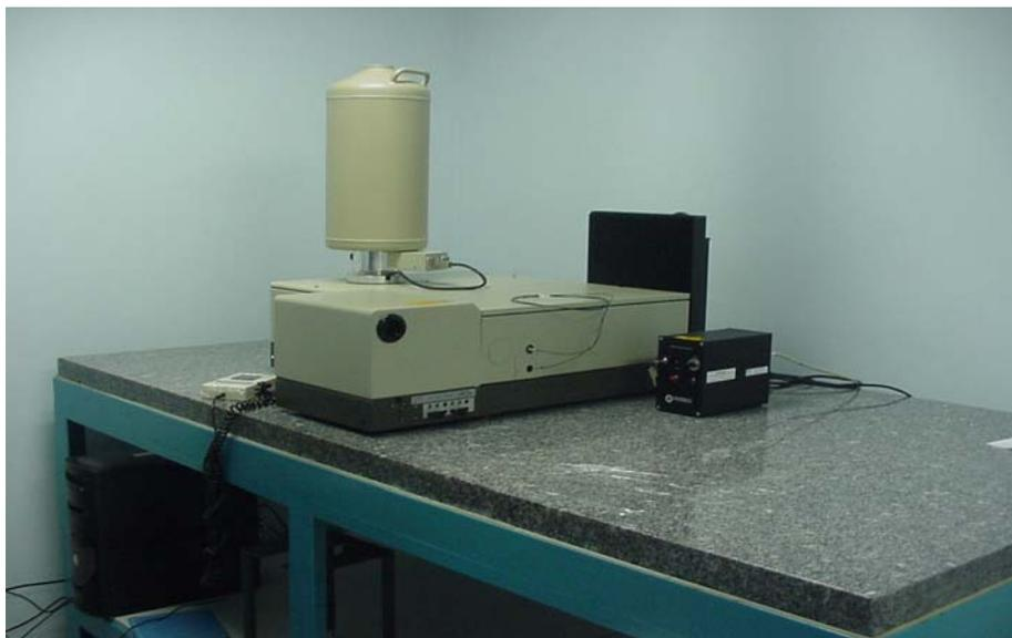
**Figura 4.** FT-Raman Spectrometer RFS 100, Bruker
