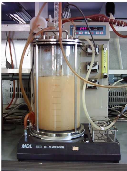
Figure 3. Stirred-tank fermentor, MARUBISHI, 8L, used for study of different aeration rates.
