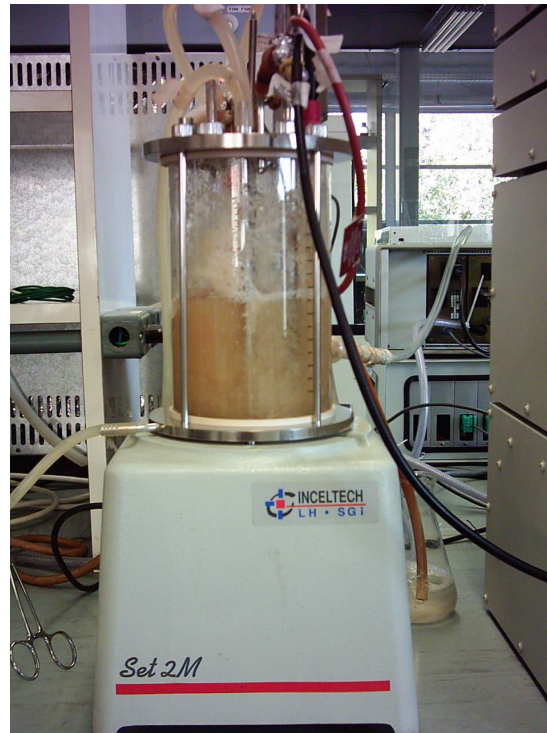
Figure 2. Stirred-tank fermentor, INCELTECH, 2L, used for the pH control studies.
