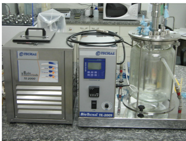
FIGURE 3 – Bioreactor BioTecnal –TE 2005, five-liter capacity.
